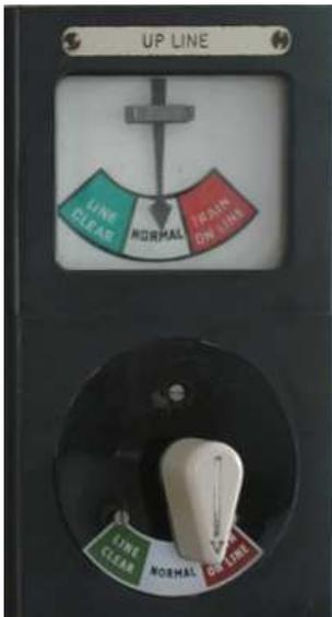
To effectively administer the block system and to allow trains to proceed from section to section without delay a strict protocol of communication was followed by signalmen. Above the familiar row of levers in a signal box stands the instrument shelf with the block instruments on it. On the front of each instrument is a dial with a lever or slide indicating three settings:
